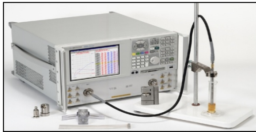
Figure 1: Agilent 85070E Dielectric Probe Kit (courtesy: home.agilent.com)
