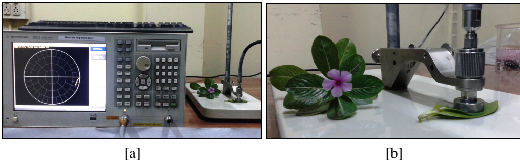
Figure 2 [a] and [b]: Dielectric Constant measurement set up for Catharanthus Roseus Leaf samples with Agilent 85070E Dielectric Probe Kit and VNA
