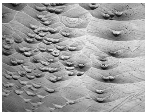
Fig.6. Observed etch pits of as grown crystal of GSN
