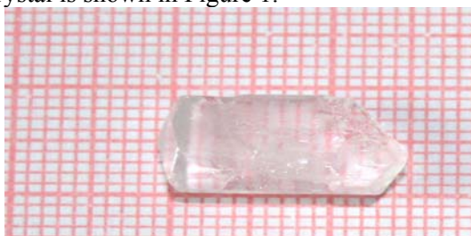
Figure 1. As grown single crystal of GG
