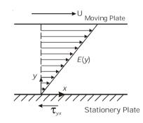
Channel walls are impermeable. Write the boundary condition for tangential and normal components of velocity at both top and bottom walls.
