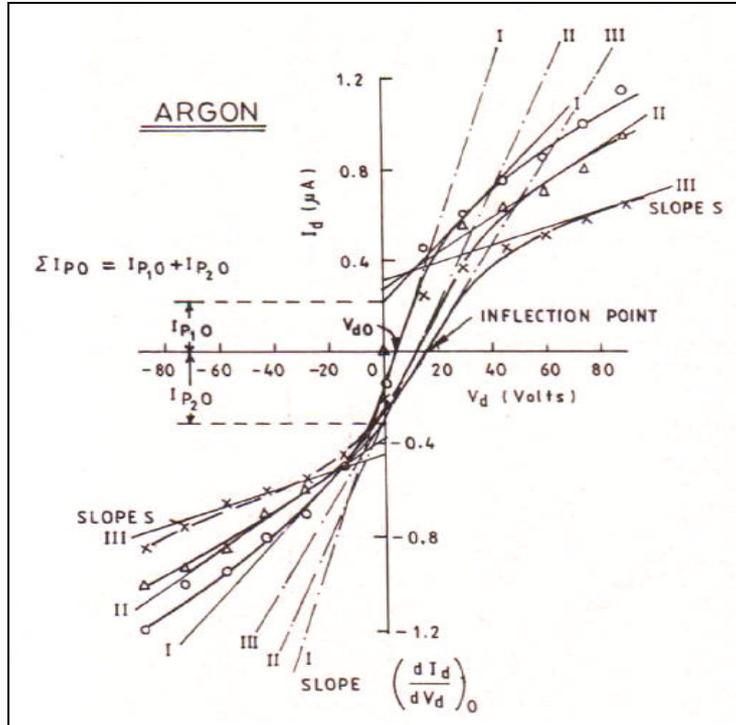
**Fig.- 2 Schematic diagram of double probe characteristics .**
