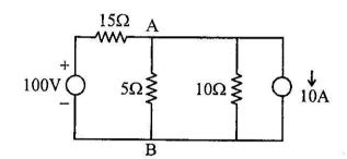
(b) In the given circuit, find the reading of the voltmeter V. Interchange, the current source and the voltmeter and verify the reciprocity theorem.
