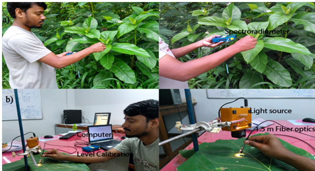
Figure 4.2: Spectroradiometry field survey (a) and laboratory analysis of collected spectra (b)
