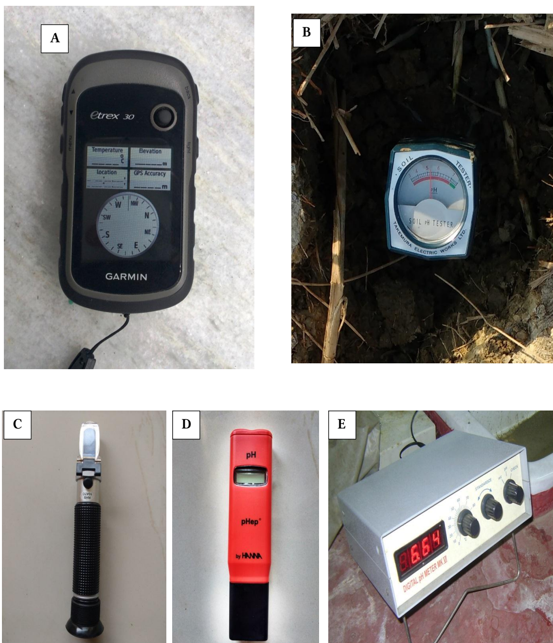
Figure 4.4 Instruments used in this study (A) Garmin GPS etrex-30, (B) Soil pH tester, (C) Hand held Refractometer, (D) Water pH meter, (E) Digital pH meter
