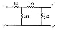
(f) When can you call a 'T-network' symmetric? Write the expression of characteristic impedance of the symmetric T-network.
