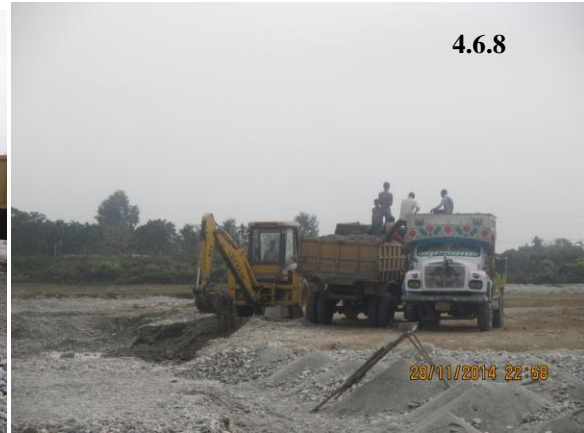
Plate 4.6.5, 4.6.6 & 4.6.7 Manual way of sediment extraction wherein crushing and segregation is done on the river bed only; 4.6.8 Mechanized sediment extractions collect large volume but crushing and segregation happens with sieves at processing units.
