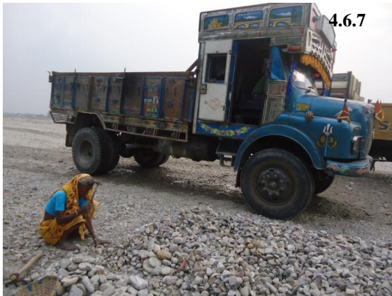
Plate 4.6.5, 4.6.6 & 4.6.7 Manual way of sediment extraction wherein crushing and segregation is done on the river bed only; 4.6.8 Mechanized sediment extractions collect large volume but crushing and segregation happens with sieves at processing units.
