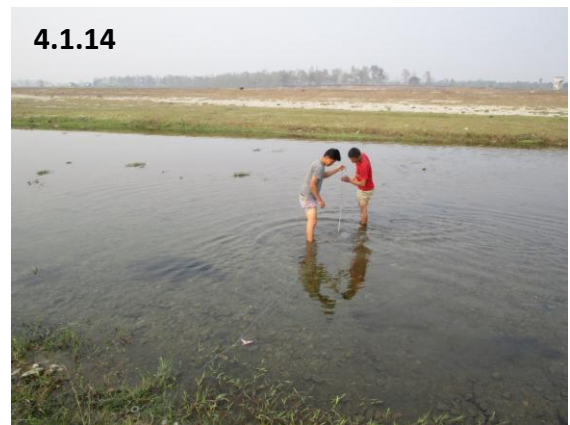
Plate 4.1.13-4.1.14 Nature of flow. (4.1.13) Super critical flow near to mountain front, wherein there are some standing waves; (4.1.14) Subcritical flow far downstream wherein waves generated by field assistants are moving upstream on the water surface.
