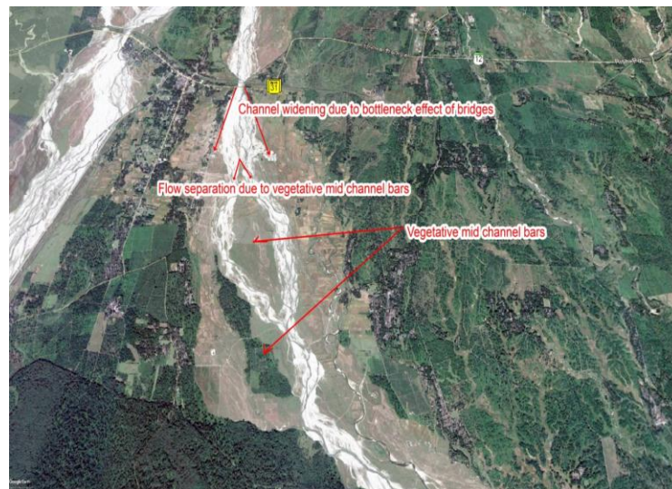
Figure 4.6.8 Channel widening due to cumulative effects of bottleneck condition and vegetative mid-channel bars in the middle reach of River Chel (Source- Google Earth Image dt. 11.07.2017).
