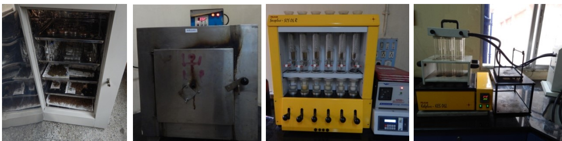
a) Hot air oven b) Muffle furnace c) lipid extraction d) Nitrogen digestion
