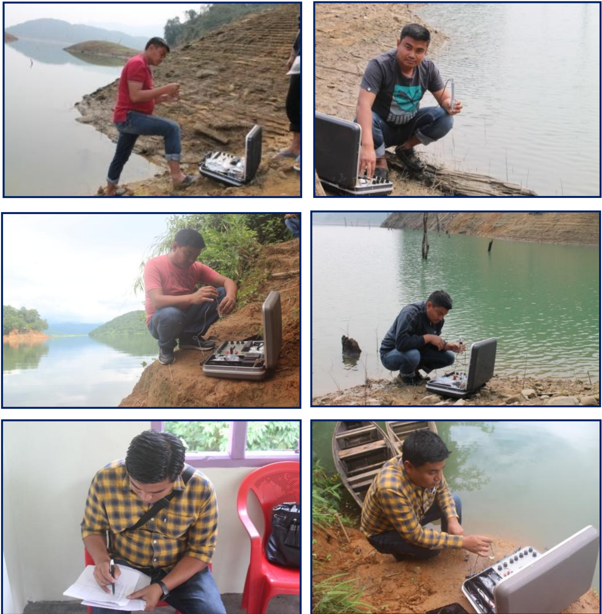
Figure 13: In-situ data collection and physico-chemical parameter analysis during different time periods from different sites of Doyang reservoir.
