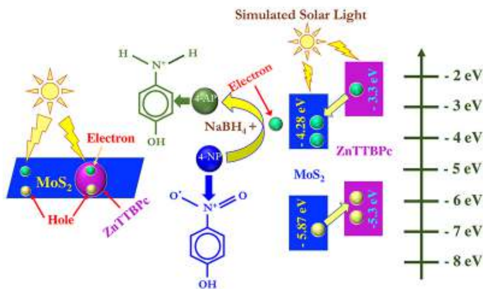
Figure 5.1.1: Photo Catalytic degradation mechanism of PNP by MoS 2 – ZnTTBPc
