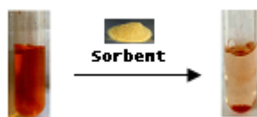
Figure 2.26 Azo dye (MO) adsorption for 48h onto network polymer matrix associated with visual color change
