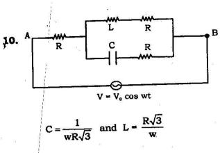
Calculate the total impedance between the point A and B.
