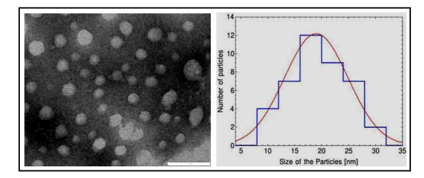
Fig 11.3. Represents the size characterization of the ECNPs using TEM studies.
