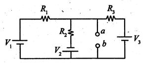
$$R_1 = 2 \Omega, R_2 = 5 \Omega, R_3 = 1 \Omega$$
