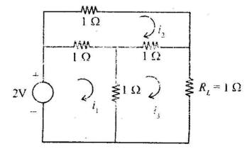
(c) For the following network, write down the tie-set matrix and determine the KVL equations. Also calculate the loop currents. 4
