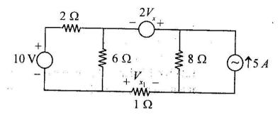
(ii) For the following network determine fundamental cut-set matrix and hence find the KCL equation.
