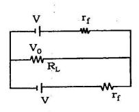
The equivalent circuit can be drawn as shown below when both the input A and B is 1, ie V volt.
