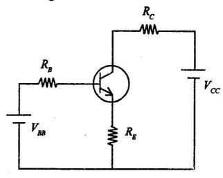
Given that  $\beta = 100$ ,  $I_{CBO} = 20 \text{ nA}$ ,  $R_C = 3 \text{ k}\Omega$ ,  $R_B = 50 \text{ k}\Omega$ ,  $R_E = 2\text{k}\Omega$ ,  $V_{CC} = 10 \text{ V}$ ,  $V_{BB} = 5\text{ V}$ ,  $V_{BE}$  (active) = 0.7 V,  $V_{BE}$  (sat) = 0.8 V,  $V_{CE}$ (sat) = 0.2 V
