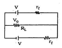
The equivalent circuit can be drawn as shown below when both the input A and B is 1, ie V volt.
