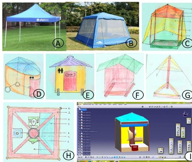
**Fig 5:** Utility and form generation exercises. (A) and (B) act as inspiration, where (C), (D), (E), (F) and (G) are the form explorations; (H) is the functional layout of different components and (I) is CAD exploration.
