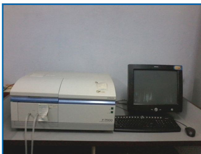
Figure 3.5: HITACHI F-7000 Fluorescence Spectrophotometer
