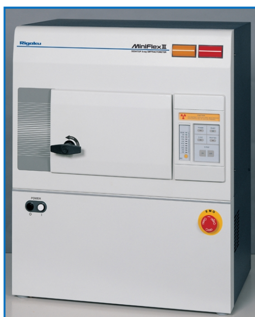
Figure 3.11: Rigaku Miniflex-II’ X-ray diffractometer
