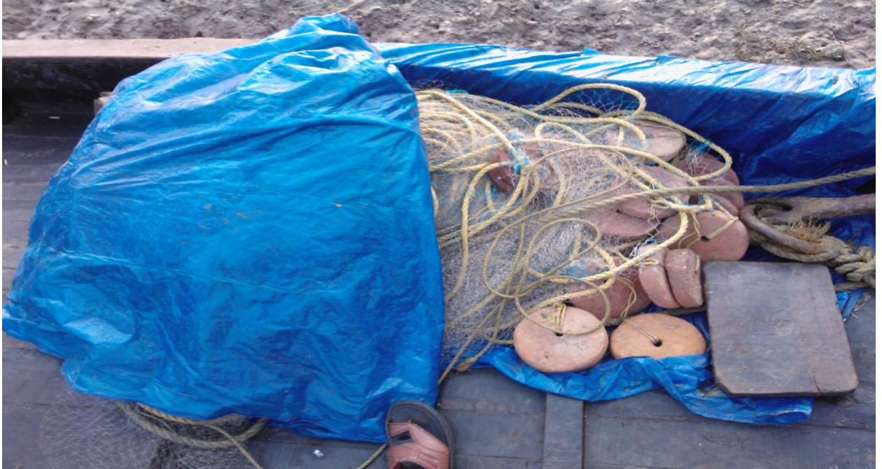
A Gill Net attached with Wheel-shaped Terracotta Sinkers.
