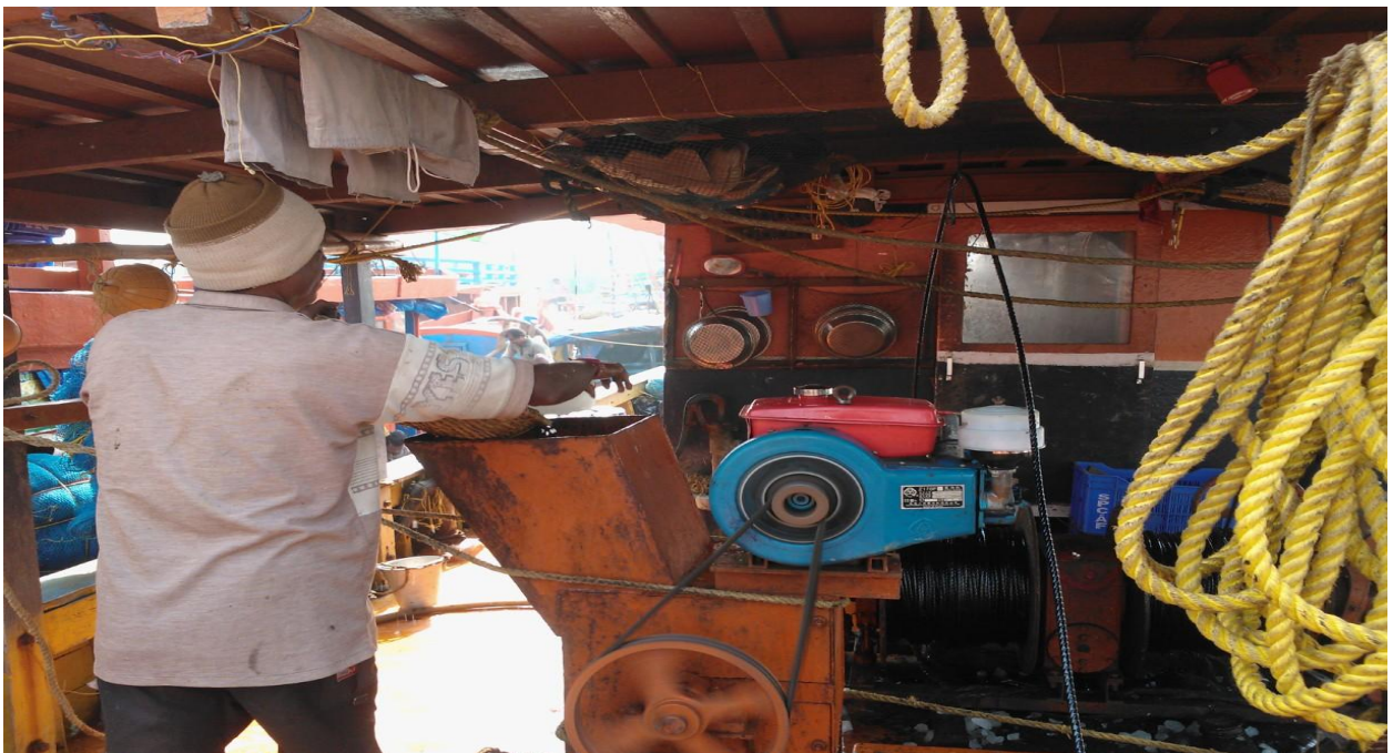
Ice Crashed on the Deck of the Vessel to Carry for Refrigeration during High Sea Fishing.
