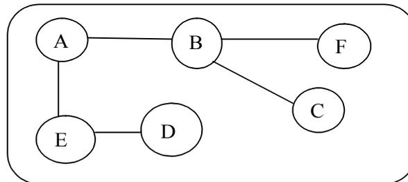
**Fig 2:** Minimum spanning tree drawn from the complete graph
