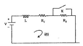
(h) Calculate the resistance R in the following circuit which will allow maximum power dissipation in it. Calculate the maximum power.
