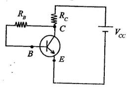
Here  $V_{CC} = 12 \text{ V}$ ,  $R_c = 1 \text{ k}\Omega$ ,  $\beta = 100$ , and  $V_{BE} = 0.7 \text{ V}$ . Find  $R_B$  which makes  $V_{CE} = 6.32 \text{ V}$ , Find also  $I_B$ , Assume  $I_{CEO} << I_B$ . 3
