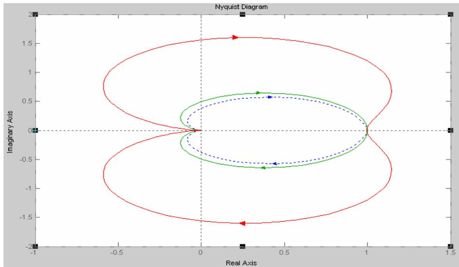
Fig. 12 Nyquist diagram for equation 15 by varying the PID coefficients
