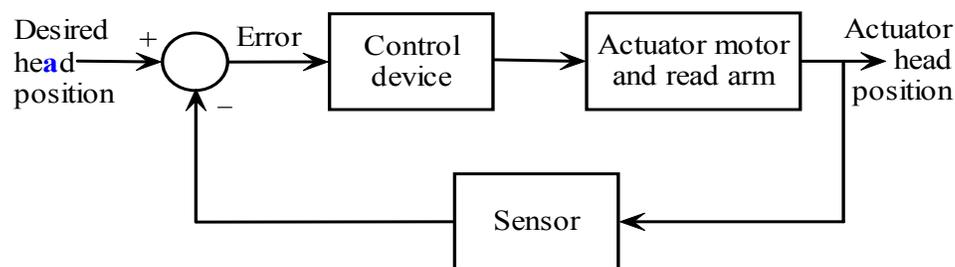
**Fig. 1: Closed-loop control system for disk drive.**
