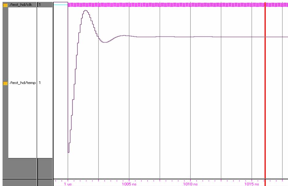
**Fig. 13 The step response of equation (16) created by ModelSim**
