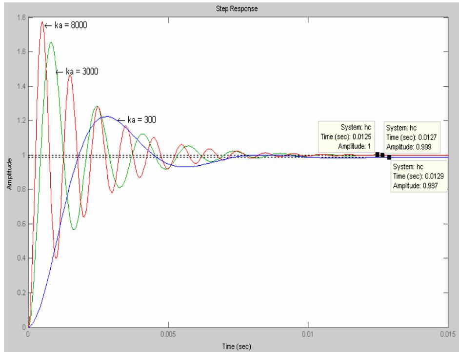
**Fig. 9** Step response to equation 3 with different values  $K_a$
