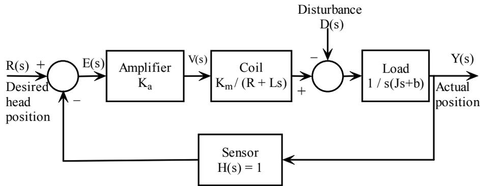
**Fig. 6: Control system for disk drive head reader.**
