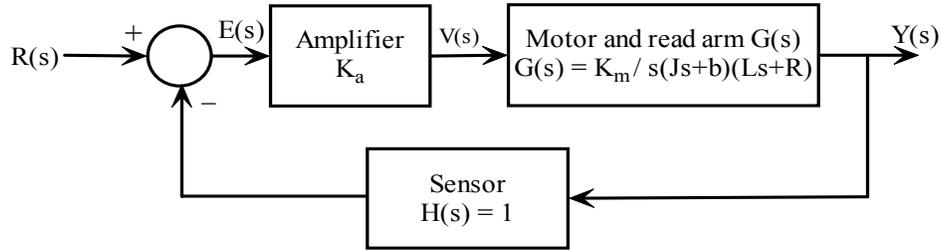
**Fig. 2: Block diagram model of disk drive read system.**
