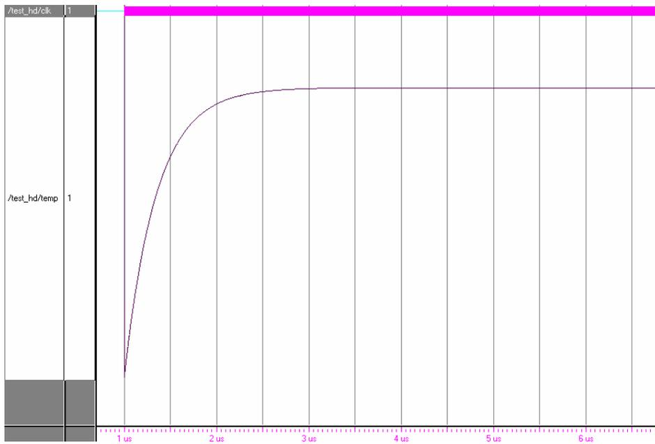
**Fig. 14** The step response of equation (19) created by ModelSim
