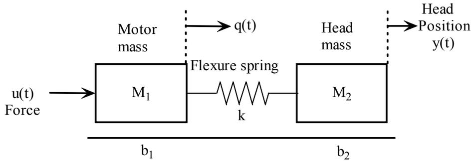
Fig. 4(a): Model of the two-mass system with a spring flexure.
