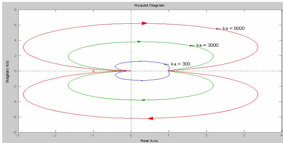
Fig. 10 Nyquist diagram for equation 3 with different values of  $K_a$
