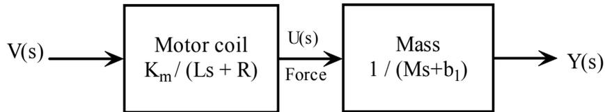
Fig. 5: Transfer function model of head reader device with rigid spring.
