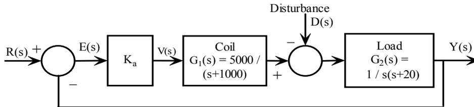
**Fig. 7: Disk drive head control system with the typical parameters.**
