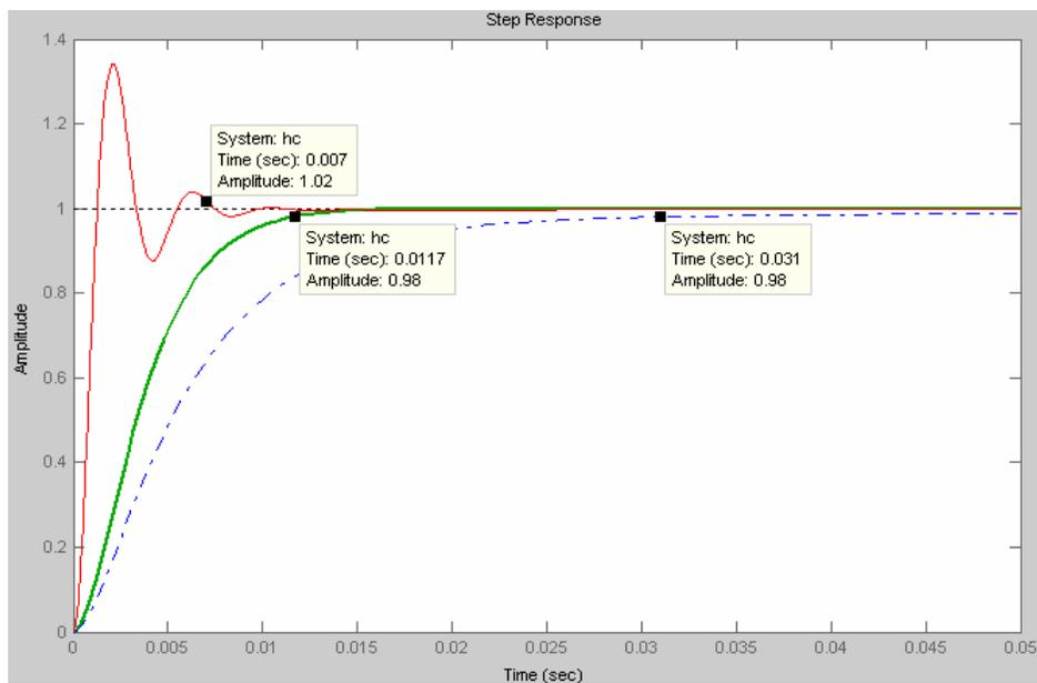
Fig. 11 : Step response to equation 15 by varying the PID coefficients
