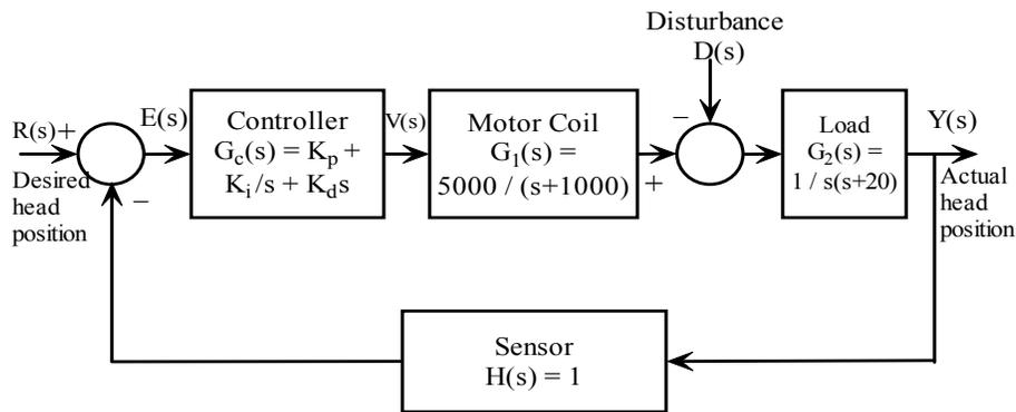
Fig. 8: Disk drive head control system with a PID controller.
