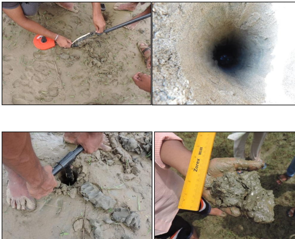
Plate 2.9, 2.10, 2.11 & 2.12: Burrowing through hand piston auger
