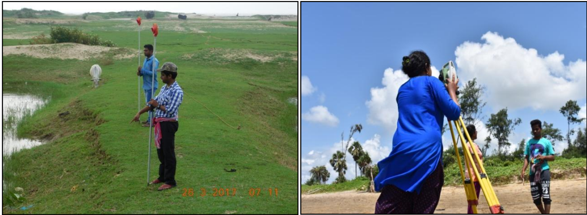
Plate 2.1 & 2.2: Total station survey
