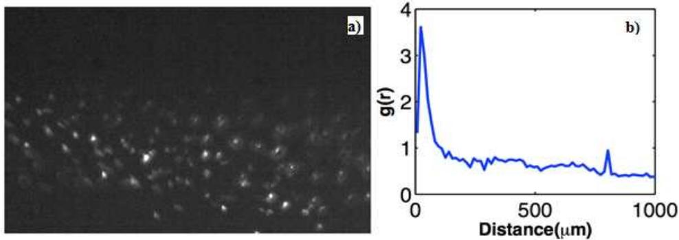
**Figure 3:** a) Image of dust cloud b) A plot of pair correlation function  $g(r)$  vs  $r$  for the eroded dust cloud of fig 3(a). The location of first peak gives the inter-particle distance.
