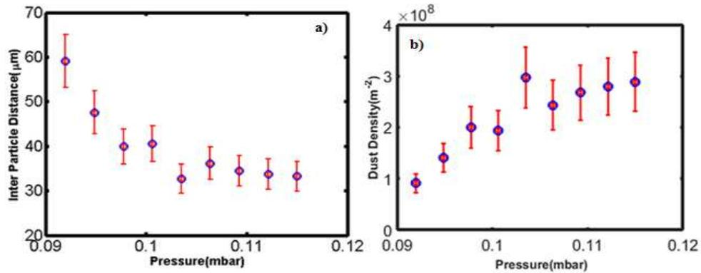
**Figure 5:** Dusty Plasma variation with neutral pressure at a fixed discharge voltage
