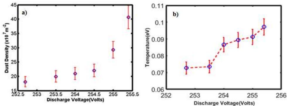
**Figure 4:** Dusty Plasma variation with discharge voltage at a fixed neutral pressure
