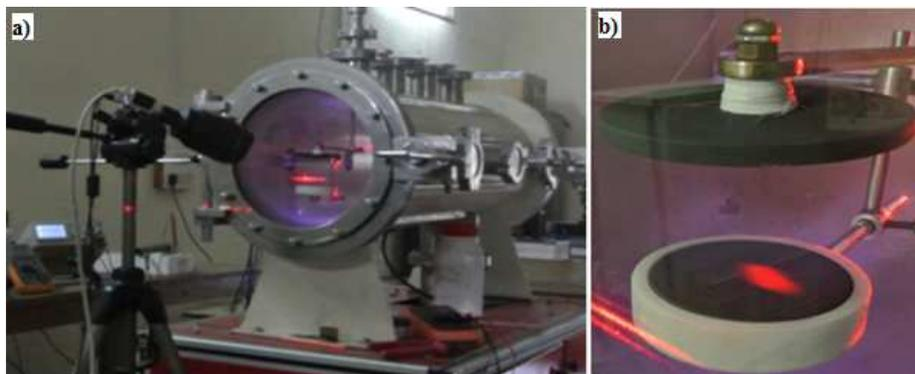
**Figure 1:** Picture of the argon plasma with carbon dust cloud in between two electrodes
