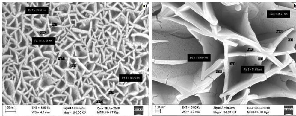
**Figure 2:** SEM Photograph of sputtered graphite cluster (a) at  $V_D = 270$  Volts and  $P = 0.085$  mbar b)  $V_D = 278$  Volts and same neutral pressure.
