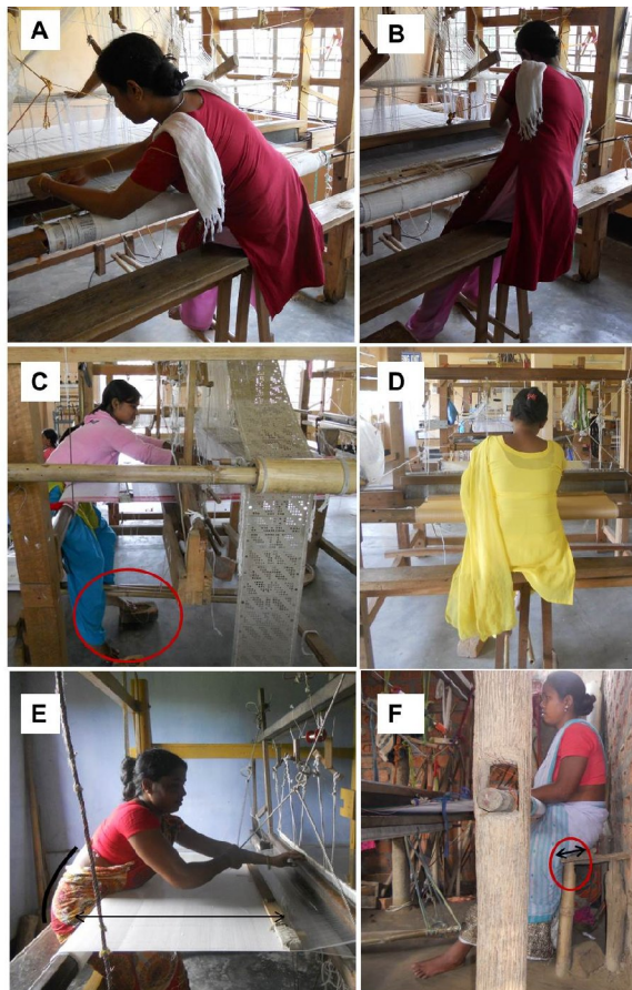
Fig 1: Showing existing seat design in different handloom industry of Assam A and B . Forward and Side bending posture to maintain thread breakage C . Legs dangling due to fixed seat height D . Upright sitting posture for continuous weaving E . Forward stretched posture F . Narrow width of the plank and sharp hard edge in front of the seat.
